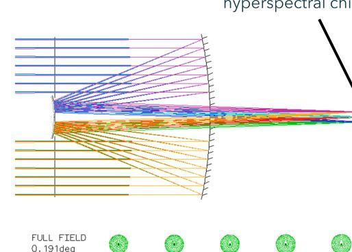
Ray trace results for an 80mm primary aperture Cassegrain telescope for CubeSat form factors.
